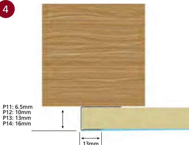
■ STOPPING BEAD DETAIL
